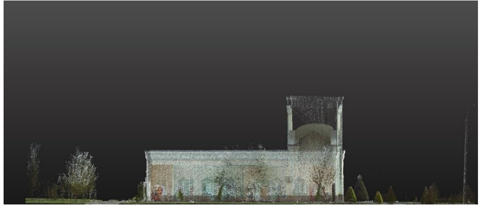
Figure 6. Side Facade of the Building Created Based on 3D Scanning.
